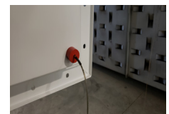
Optional SmartBatch part temperature monitoring
